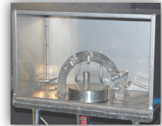
Figure 2. Spray nozzle configuration for IP69K capable simulation systems and image of actual spray system.
